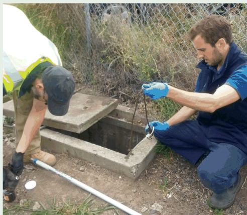
Figure SP6: Stormwater runoff drainage pit sampling
