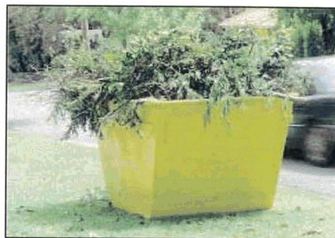
An incorrectly loaded waste bin.
