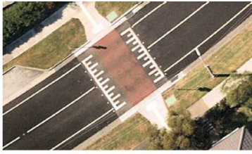
RAISED SAFETY PLATFORM AND PEDESTRIAN CONNECTIVITY IMPROVEMENTS
