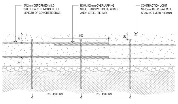
REINFORCED CONCRETE EDGE DETAIL **DETAIL CROSS SECTION**
