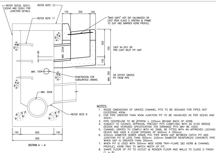
DOUBLE CHANNEL GRATED PIT HB2/B2 KERB & CHANNEL
